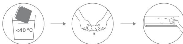
Figure 9 — Cleaning the indoor unit housing
