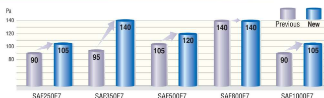
Increased external static pressure at UHi air flow
