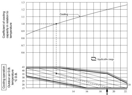
Indoor air W.B. temperature °C W.B. ISO-T1 Standard Condition
