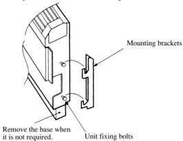
Note (1) The figure on the left shows the wall mounted installation when the base is removed.
