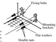
Install the suspension brackets so that this plane will be level or will have a gentle incline toward the right. (left and right side height difference should be from 0 to 0.1 in.)
