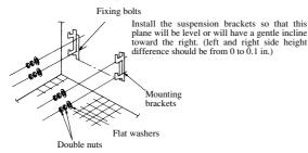
Note (1) Location of the mounting brackets fixing bolts are the same as those for the floor standing installation except the location height.
