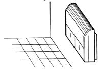
4) Fix the unit on the floor by using the fixing brackets.
