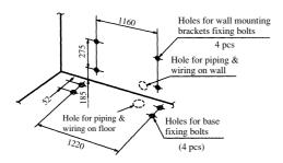
Fix the mounting brackets on a wall.
